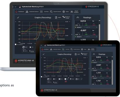
Data can be viewed in graphical or numerical format and recorded data can be exported in PDF or CSV format. During tests graphical data can be interrogated by zooming and also adding annotations.
