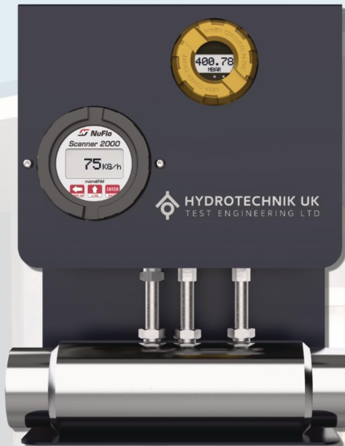
A cutting-edge flow meter designed specifically for use with hydrogen but also available for other gases such as nitrogen, air or natural gas on request. Flow rate, static pressure and temperature values are accessible via the built-in display and, optionally, via the built-in Modbus connection.
