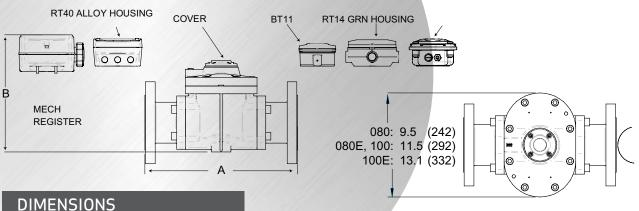
All dimensions are inches ± .079" (millimeters ±2mm)
