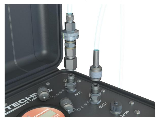
To disconnect the hoses, unscrew from the Minimess Test Point. The hose assemblies do not contain a self-seal mechanism and may drip; keep an oil absorbent spill mat ready and store hoses in a plastic bag when not in use.
