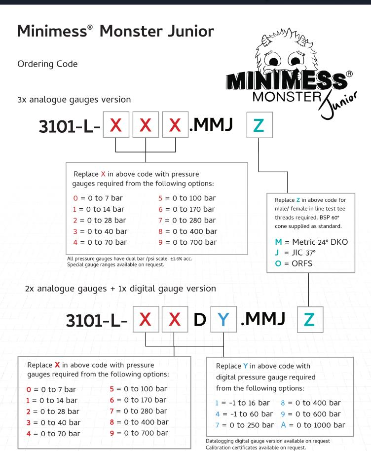
All pressure gauges have dual bar/psi scale.±1.6% acc. Special gauge ranges available on request.
