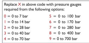
All pressure gauges have dual bar / psi scale.  $\pm$  1.6% acc. Special gauge ranges available on request
