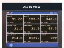
View up to 42 channels of data as graph, alphanumeric or display tiles with easy viewing page by page.
