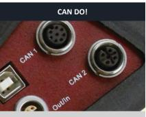
2 baud rate independent CAN lines for increased CANbus sensor, calculations or system J1939 measurements.
