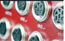
8x high speed (up to 0.1ms) measurement channels. 2x selectable analogue or frequency channels allow more flexibility.
