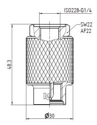
This adapter is suitable to connect pressure sensors, hose assemblies or other components with ISO228- G1/4 Type F stud end.
