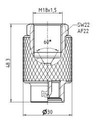
This adapter is suitable for connecting pressure sensors or other components with M18x1.5 screw-in stud and 58° sealing cone.
