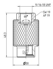
This adapter is suitable for connecting pipes, hose lines or other components with 1/4" - 58° sealing cone and 9/16"-18 UNF threaded stud.
