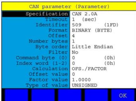
All parameters must be defined exactly like shown, otherwise there will be no communication. Specific for the size class ISO 4 µm are the options „Identifier“ and „Offset“. For ISO size classes you should enter an identifier resulting from the addition of the Patrick Node-ID (see type plate or Patrick operation menu) plus 384 (here Node-ID 125: identifier = 125 + 384 = 509). For SAE size classes you must add 640 to the Patrick Node-ID.
