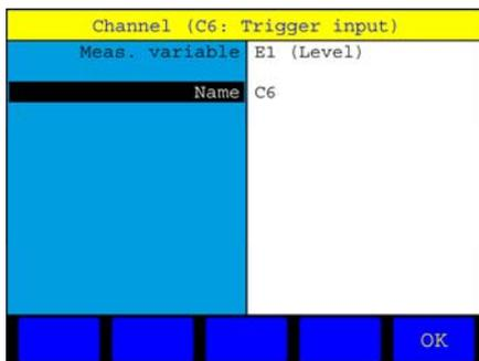
You may feed an external signal via the trigger input channel into the instrument to start a recording. Please see section 3.2.4 on page 9 for information on allowed trigger signals.
