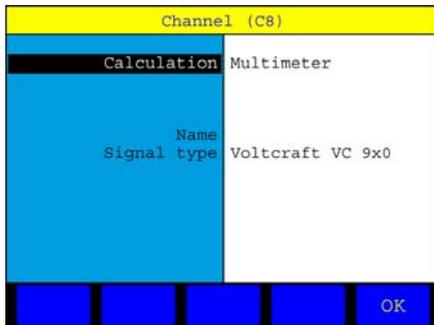
Here you may assign a name to the channel and select the type of the connected Multimeter. Currently the types Voltcraft VC 820, VC 920, 940 and 960 are supported.
