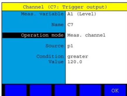
The trigger channel may be used to start a simultaneous recording on connected instruments. Please see the section "Simultaneous recording on connected instruments" on page 26.
