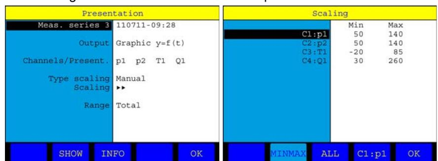
put the option „Type scaling“ to „Manual“, highlight the option „Scaling“ and press **ENT**; highlight a channel, press **ENT** and input the start and end value of the data range that shall be presented
