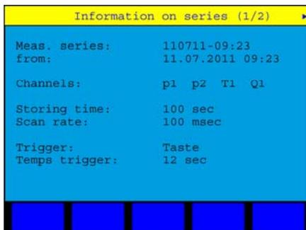
Here you can see the available information on the measuring series. The trigger time shows, how much time expired after starting the recording before the trigger event happened. Press
