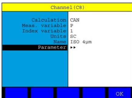
The calculation is CAN, since Patrick sends the data via CAN bus. The variable P stands for particle, the index is 1 for particle size class ISO 4 µm, what is used as name, too. You have to enter a name as units, here “SC” (= size class).
