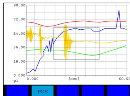
a rectangle is shown in the center of the diagram; this shows the area that will be enlarged; since **F2** is occupied with the function „POS“ you may use the arrow keys to shift the rectangle; then press **F2** to switch to „SIZE“; now you may use the arrow keys to change the size of the rectangle; press **ENT** to apply the zoom:
