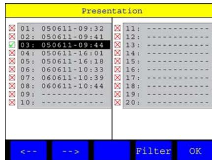
Highlight the desired measurement series and press **F5**. Use **F1** / **F2** to scroll through the pages of the list. Press **F4** to sort the list:
