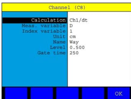
You may use this function e.g. to calculate speed from a measured way. You may define a threshold value (“Level”) to prevent the calculation of absurd values for small way measurements. This assures that a certain way has to be measured before a calculation is executed. The gate time assures for a defined level that a calculation is executed after a certain time. This is the only way to assure the calculation of a speed “0”.
