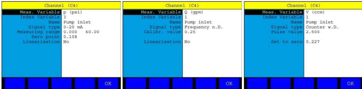
The combined input channels can be used for sensors with analog or frequency output signal. The channel is set by selecting the appropriate signal type.
