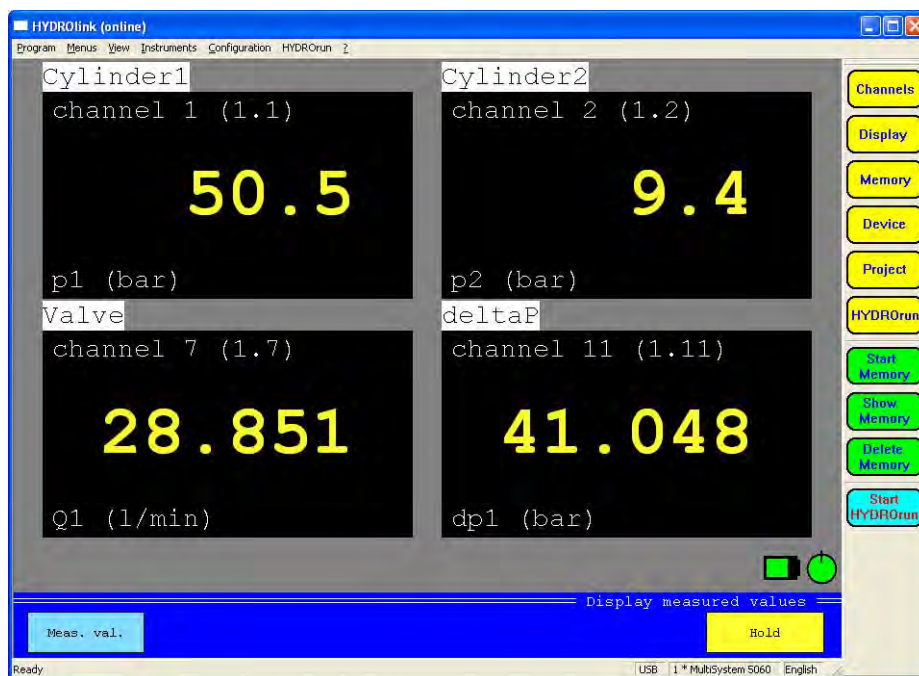
Pic. 4 HYDROlink online screen (text mode – measured values)
