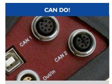
2 baud rate independent CAN lines for increased CANbus sensor, calculations or system J1939 measurements.
