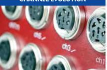
8x high speed (up to 0.1 ms) measurement channels. 2x selectable analogue or frequency channels allow more flexibility.
