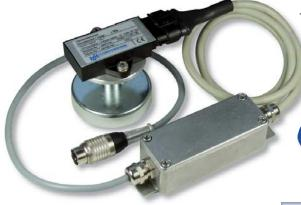
The vibration sensor comprises a capacitive acceleration sensor for data collection with short response time under serious environmental conditions. It is mounted on a magnetic foot that can be used to attach the sensor to any metallic surfaces. It reports vibrations by frequency and therefore can be connected to all Hydrotechnik measuring instruments.
